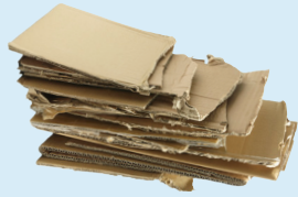
Corrugated Cardboard (Wavy center layer)
